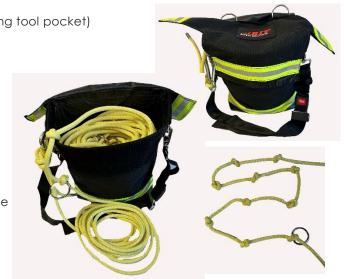
Specs: Outside carabiner (snaphook) first ring (steel ring) indicates 20ft. with one knot, second ring (steel ring) indicates 40ft, with two knots, third ring (steel ring) indicates 60 ft. with three knots. Rope tied to the snap hook and attached to the bottom of the bag (Kevlar 3/8th rope).
