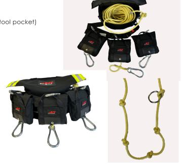
Specs: Outside carabiner (snap hook) first ring (steel ring) indicates 20ft. with one knot, second ring (steel ring) indicates 40ft, with two knots, third ring (steel ring) indicates 60 ft. with three knots. Rope tied to the snap hook and attached to the bottom of the bag (Kevlar 3/8th rope).
