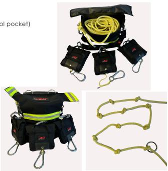
Specs: Outside, anchor point carabiner (snap hook) first ring (steel ring) indicates 20ft. with one knot, second ring (steel ring) indicates 40ft, with two knots, and third ring (steel ring) indicates 60 ft. with three knots. Rope tied to the snap hook and attached to the bottom of the bag (Kevlar, 3/8th rope).
