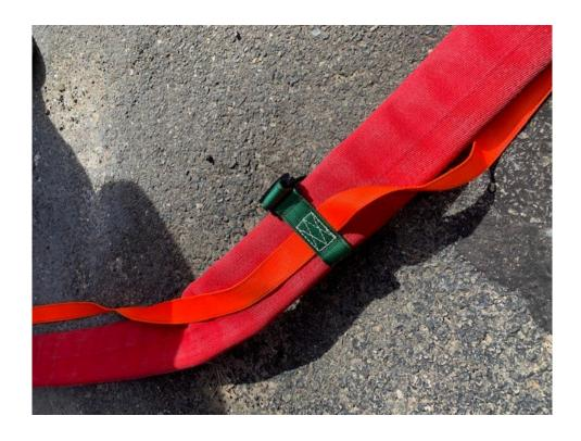
The end of the hose with the 3 black tethers goes on the pump panel. Notice there is extra slack on tether that connects to the panel side. This is intended to ensure the connection if the line does not play out correctly.
